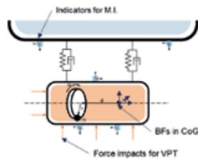
Schematic drawing of the ELAC mounted condition for the in-situ blocked force characterization.
