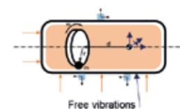
Schematic display of the ELAC freely suspended condition for In-Situ blocked force characterization.
