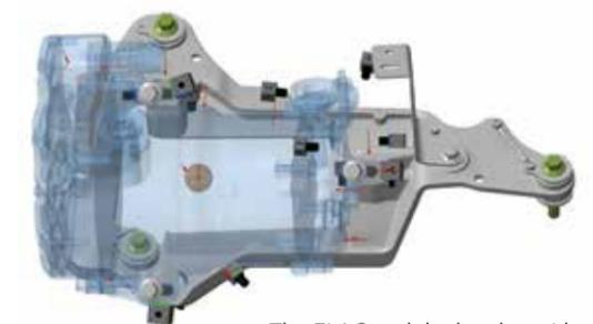
The ELAC and the bracket with a virtual point in the center of gravity.
