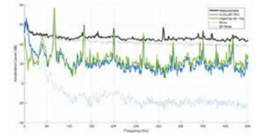
Comparison between the measured signal and the predictions from the blocked forces obtained from the freely suspended condition (green) and the mounted condition (blue).
