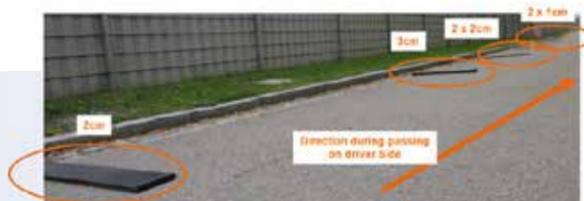
The photo shows the test track for the one sided drive over of the rubber mats with different thicknesses.
