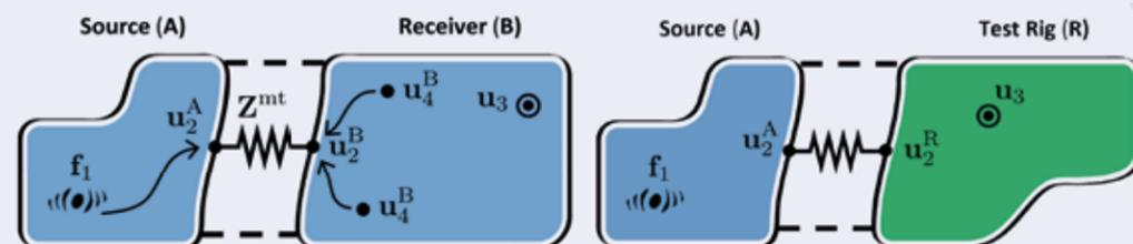
The organization of the modules in SOURCE closely aligns with the process of the TPA framework. SOURCE is designed to set up several analysis types quickly and cross-validate the results of methods from different TPA families. Intermediate results, such as force characterizations are all accessible as well. SOURCE can be used to apply any of the presented methods from the classical, component and transmissibility-based TPA families.
