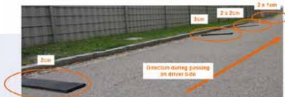
The photo shows the test track for the one sided drive over of the rubber mats with different thicknesses.
