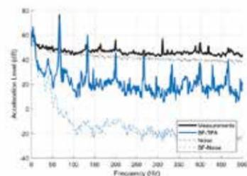
The on-board validation for the seat rail sensor. The results are shown for the state at 4000 RPM.
