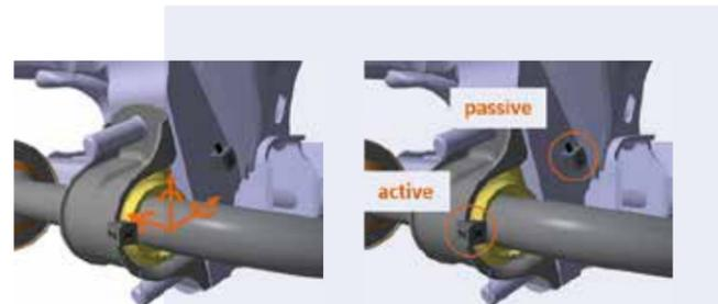
Screenshots from DIRAC. The left shows the virtual point transformed approaches for 3-DoF and 6-DoF calculation. The right shows the approach where no virtual point transformation was used.
