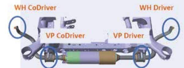
The ERC mounted to the subframe. The four virtual points are shown indicated by the blue circles.
